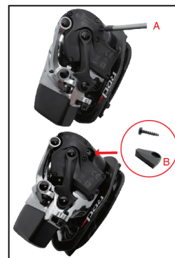
2 Use T7 star key wrench to remove rear triangular plate of rear derailleur cage. PS. A: T7 Star key wrench B: Triangle plate
