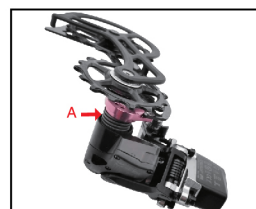
7 A: First, fix RIDEA RD5 rear derailleur cage into the body. Please do not press to the end, and reserve the space for rotating.
