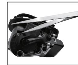
3 Use sharp tweezers or other tools to take out the tenon. Please be careful to avoid the tenon jumping. PS. Beware of tenon jumping
