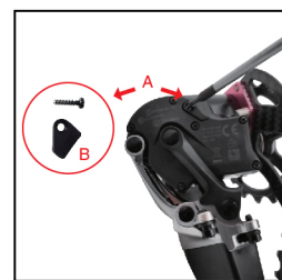
10 Assemble rear triangle plate, use T7 Star key wrench to tighten the screw on triangle plate lightly. (Please do not overtighten, or the screw may get stripped.) PS. A: Torx screw B: Triangle plate
