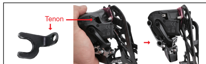
9 Assemble the tenon. Please hold the cage when assembling the tenon.
